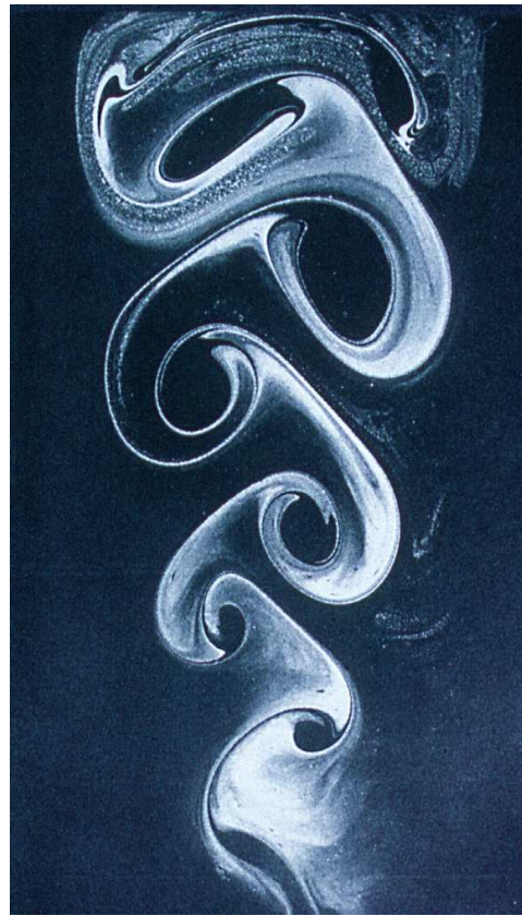
Fig. 3 This flow-pattern was created by moving a stick in a straight line from bottom to top in slow, even motion through a basin filled with water (and a substance which makes the movement visible).
